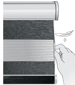
Figure 13: Correcting unaligned fabric
